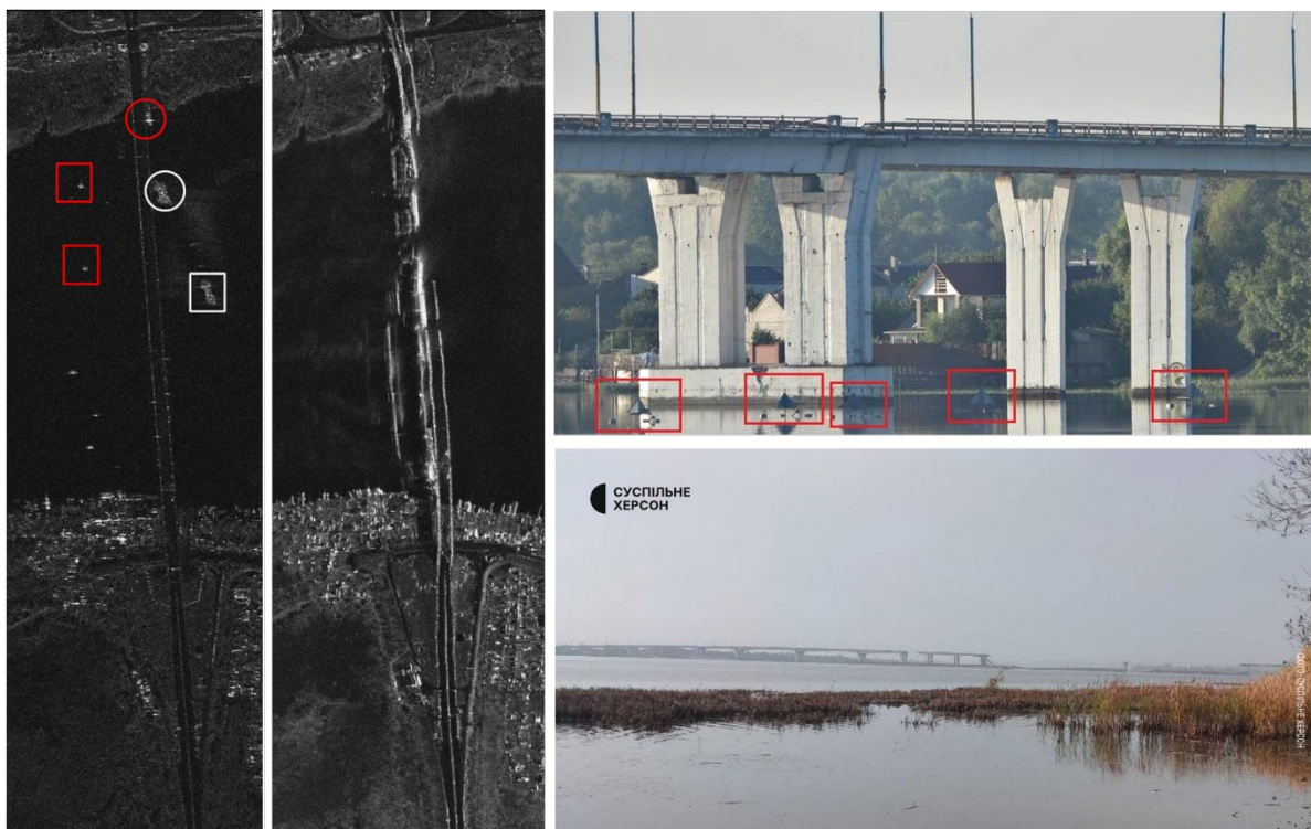
Picture n. 4: The two images on the left are high-resolution SAR imagery acquired on different days. In the first image, various targets can be identified over the river. In the second image, damage to certain parts of the bridge is visible. On the right side there are images retrieved from online newspapers, depicting the presence of floating radar reflectors and the partial collapse of the bridge. This OSINT information were essential for classifying the targets and features visible in the SAR images.
